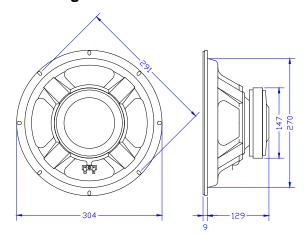
Baffle opening diameter front mounting 273 mm
