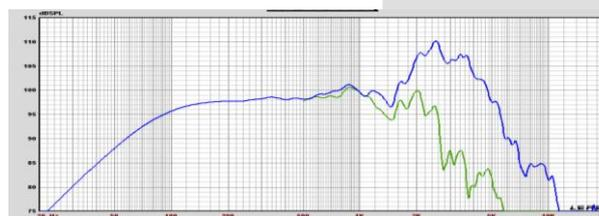
Infinite baffle sound pressure response recorded at 2.83V at one meter.
