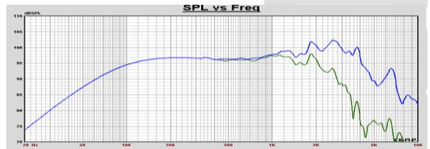
Infinite baffle sound pressure response recorded at 2.83V at one meter.
