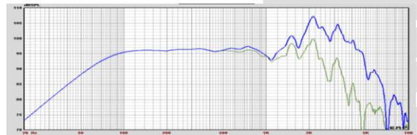
Typical infinite baffle SPL response recorded at 2.83V at one meter.
