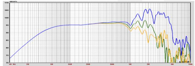
Infinite baffle sound pressure response recorded at 2.83V or nominal one watt at one meter.
