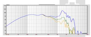
Infinite baffle sound pressure response recorded at 2.83V at one meter.
