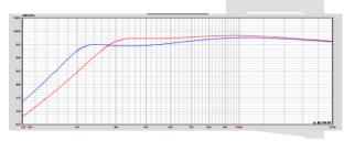
LEAP5 half space simulated vented spl response at 2.83V/1W at one meter for:
